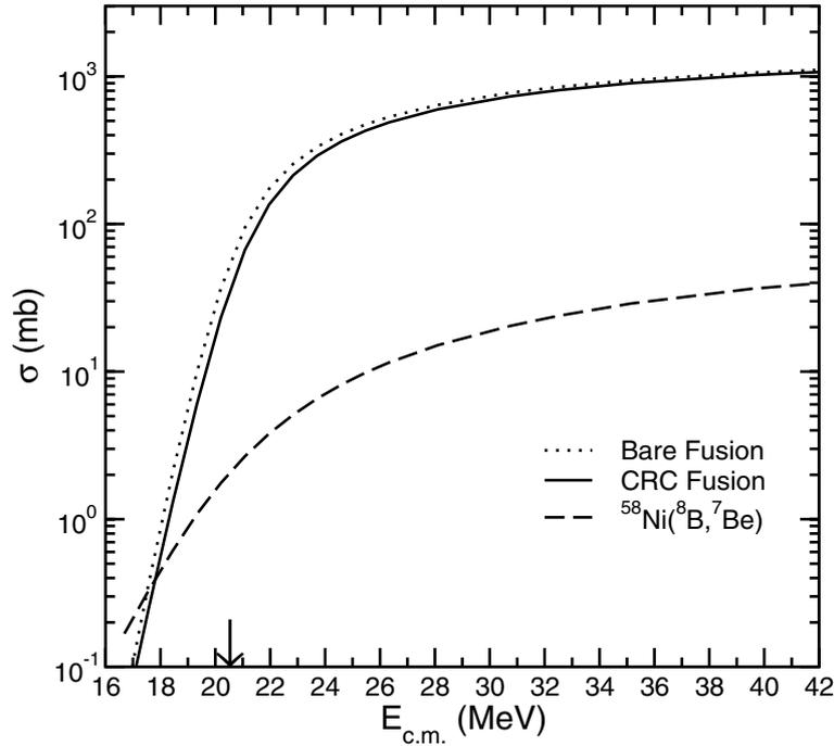
Figure 5. Total fusion cross sections with (full curve) and without (dotted curve) coupling to the  $^{58}\text{Ni}(^8\text{B}, ^7\text{Be})^{59}\text{Cu}$  stripping reaction. The dashed curve denotes the integrated stripping cross section. The arrow indicates the position of the nominal Coulomb barrier.
