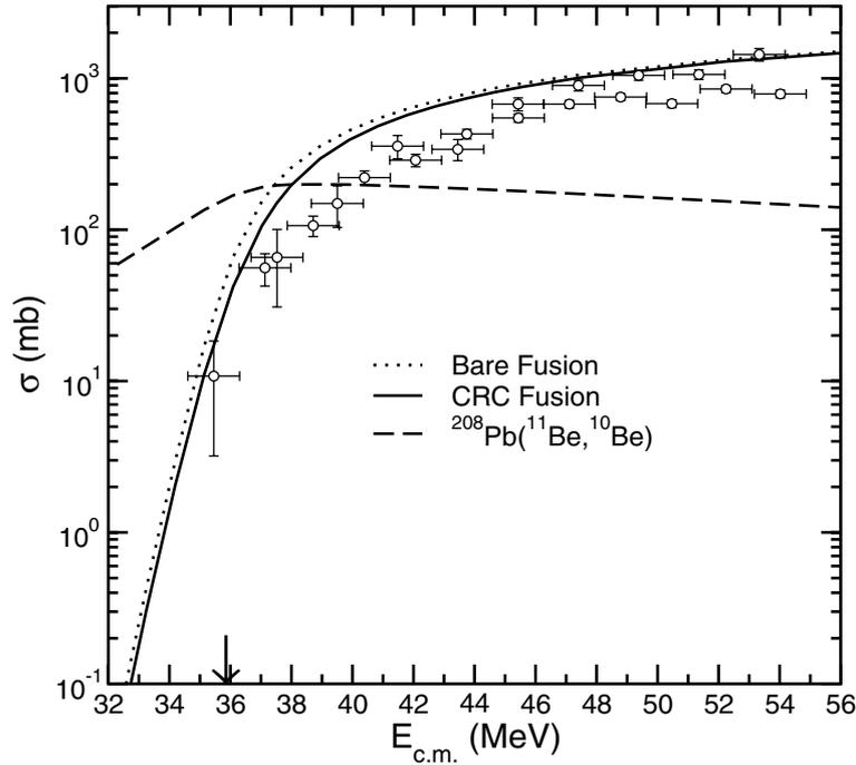
Figure 4. Total fusion cross sections with (full curve) and without (dotted curve) coupling to the  $^{208}\text{Pb}(^{11}\text{Be}, ^{10}\text{Be})^{209}\text{Pb}$  stripping reaction. The dashed curve denotes the integrated stripping cross section. The open circles denote the  $^{11}\text{Be} + ^{209}\text{Bi}$  total fusion data of [25], with the shift in Coulomb barrier height compensated for. The arrow indicates the position of the nominal Coulomb barrier.
