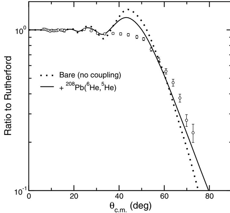
Figure 3. Elastic scattering angular distribution for 27 MeV  ${}^6\text{He} + {}^{208}\text{Pb}$  with (solid curve) and without (dotted curve) coupling to the  ${}^{208}\text{Pb}({}^6\text{He}, {}^5\text{He}){}^{209}\text{Pb}$  stripping reaction. The data are taken from [24].
