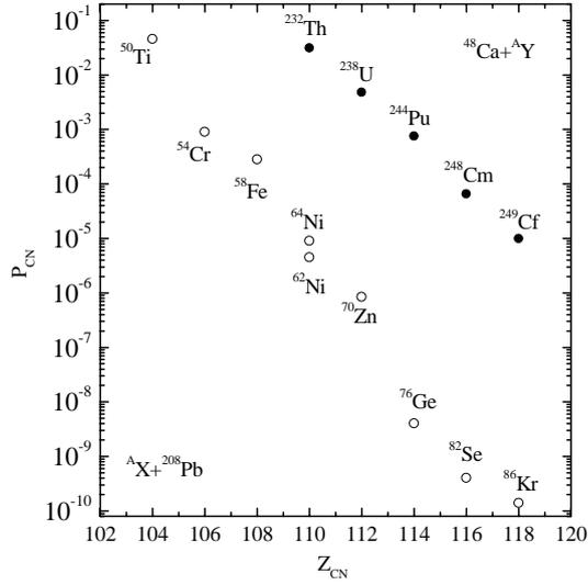
Figure 5. Calculated fusion probabilities  $P_{CN}$  for cold fusion reactions ( $^A\text{X} + ^{208}\text{Pb}$ ) and hot fusion reactions ( $^{48}\text{Ca} + ^A\text{Y}$ ) as a function of the charge number  $Z_{CN}$  of the superheavy compound nucleus.
