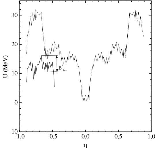
Figure 4. Potential energy of the dinuclear system in the reaction  $^{54}\text{Cr} + ^{208}\text{Pb} \rightarrow ^{262}\text{Sg}$  reaction ( $|\eta_i| = 0.59$ ) as a function of  $\eta$  for  $J = 0$ . Both curves are obtained with experimental binding energies. The dotted curve is calculated for spherical shapes of the nuclei, the solid curve for deformed shapes in pole-to-pole orientations.
