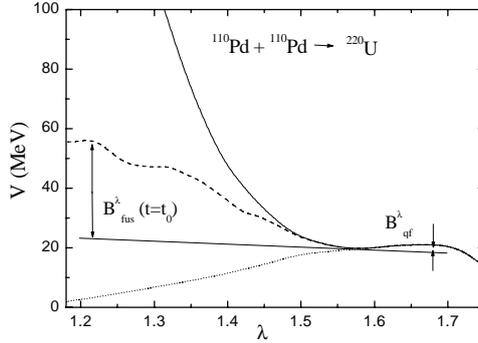
Figure 2. The diabatic (solid curve), the diabatic time-dependent (dashed curve) and the adiabatic (dotted curve) potentials for  $^{110}\text{Pd} + ^{110}\text{Pd}$  as a function of  $\lambda$ .
