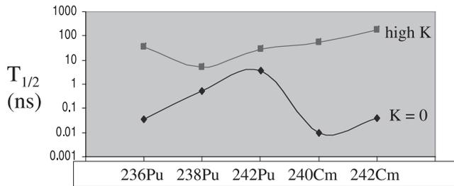
Figure 1. Half-lives of fission isomers in even-even nuclei. The label “K = 0” refers to the lowest-energy state in the second well, and “high K” refers to the excited isomer in the second well. The data are from Bjørnholm and Lynn [12].
