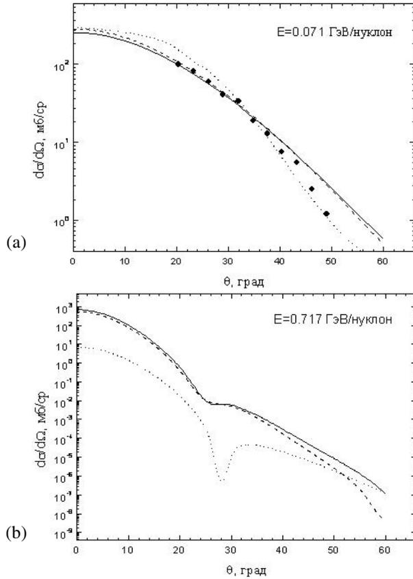
Figure 1. The calculation of DCS with different model wave functions: the solid and dotted curve – ann wave function in models 1 and 2, dashed curve – oscillator wave function, with: (a)  $E = 0.071$  GeV/nucleon, the experimental points from [13], (b)  $E = 0.717$  GeV/nucleon, the experimental points from [1].
