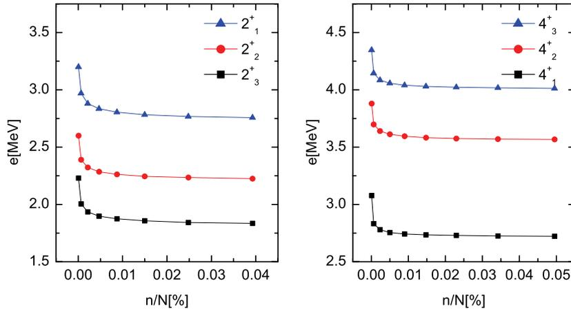
Figure 2. Convergence rate of the lowest  $J^\pi = 2^+$  and  $4^+$  energy levels in  $^{96}\text{Zr}$ . The  $n/N$  variable is the ratio between the dimensions of the sampled over the full space
