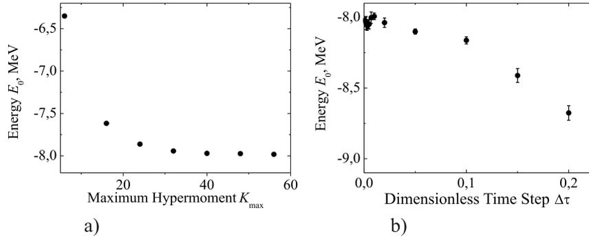
Figure 1. The convergence of HHMS (a) and FCI (b) algorithms for the model of a 3-body system with nuclear interaction (28); the exact value of the ground state energy is  $E_0 = -8$  MeV.
