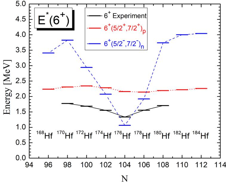
Figure 1. Theoretical  $K^\pi = 6^+$  excitation energies from neutron (blue level-bars) and proton (red bars) 2q.p. configurations obtained for the  $^{168-184}\text{Hf}$  isotopic chain compared with experimental data [2]. See the text for details.
